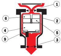
Simultaneous drainage of liquid from Valve Chamber (2) causes Floats (4), (5) and (6) to gravitate downwards into the Baffle Plate (9), thereby allowing atmospheric air through the valve to rapidly displace draining liquid in the pipeline and prevent potentially damaging internal negative pressure..
