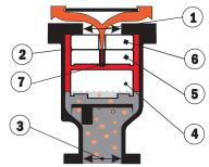
Subsequent to the filling of a pipeline, liquid enters the valve Barrel Chamber (2) and the Floats (4), (5) and (6) are buoyed so that the Large Orifice (1) is closed by Float (6). The valve will then become internally pressurised. A minimal working pressure of < 0.5 bar (7.3 psi) acting on the relatively large area of the Orifice (1) will lock Float (6) into the closed position across the Large Orifice (1).
