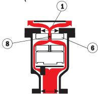
In reaction to increased air flow, Float (6) closes Large Oriface (1) and air is forced through the Anti Shock Oriface (8) resulting in deceleration of the approaching water due to the resistance of rising air pressure in the valve.
